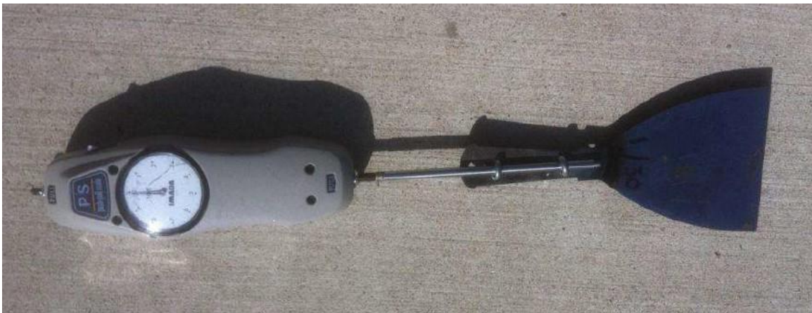
Figure 1.8. Custom BHG created by Buhler to measure snow hardness (Buhler, 2013).
