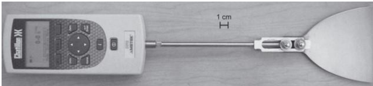
Figure 1.7. First iteration of the BHG designed by Chris Borstad and David McClung (Borstad & McClung, 2011).
