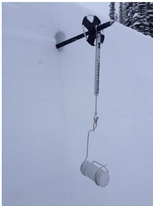
Figure 2.12. Snow density apparatus including the Pesola Scale and 100 cm 3 metal cylinder (photo by author).
