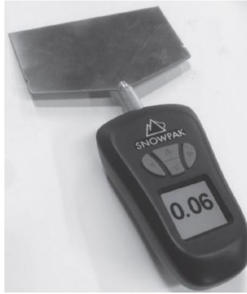
Figure 1.10. Blade Hardness Gauge produced by Fraser Pogue in 2017 (Pogue et al., 2018).
