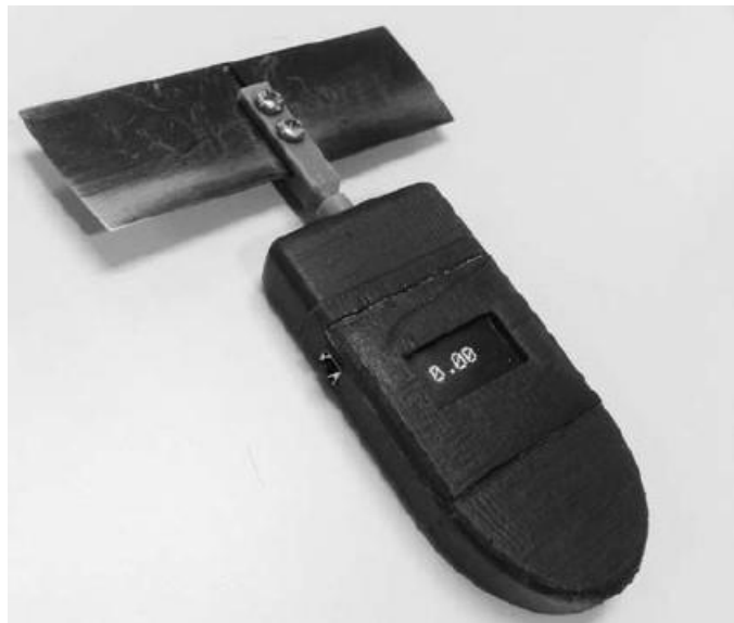
Figure 1.9. Blade Hardness Gauge produced by Fraser Pogue in 2016 (Pogue & McClung, 2016).
