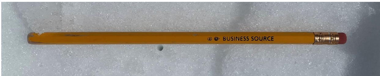
Figure 2.13. Standard pencil used during the hand hardness test (photo by author).
